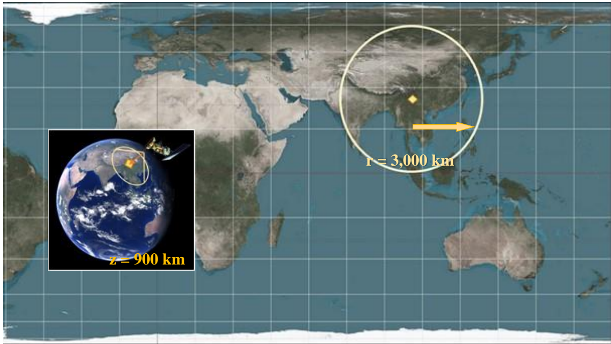
Figure 3.8: Footprint of LEOSAR Satellite (Sarsat-10)
